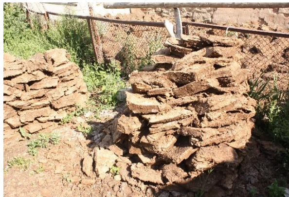
Figure 19: Dung bricks stacked to dry
