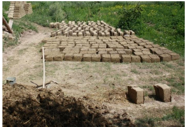
Figure 13: kirpitsch bricks being made. Front: mixture of clay and straw, back: bricks laid out to dry
