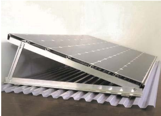
Figure 6: Modified sub-construction based on a Tritec mounting system for corrugated metal roofs. The sub-construction is adapted to the mounting of a SUC-module with rear side aluminum beams. In this example a frameless glass/backsheet with 0.8 mm glass thickness has been applied.
