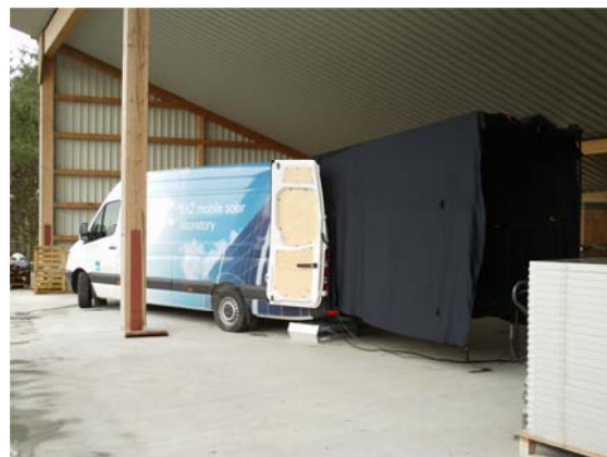
Figure 1: The Swiss Mobile Flasher Bus in operation at a customer site in Southern Germany in Dec 2009. The Bus is equipped with a high accurate Flasher from Pasan.
