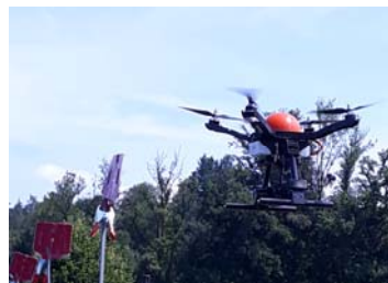
Figure 4. RotorKonzept RKM 4X UAV equipped with a Sony DSC-RX100M4 camera taking photos of sticky traps.
