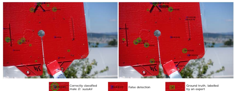
Figure 5. AlexNet (left) and GoogLeNet (right) classifiers applied to detect D. suzukii fruit flies in a sticky trap. The image was taken with a Sony DSC-RX100M4 mounted on a RotorKonzept RKM 4X UAV (figure 4). Initial proposal locations were determined using the SelectiveSearch 3 algorithm.
