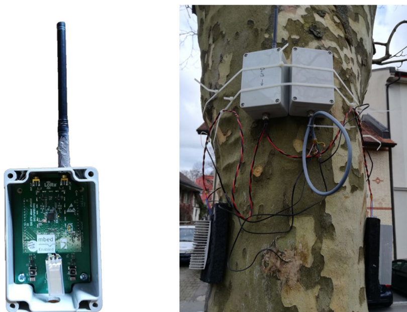
Fig. 2 The embedded system powered by EH is fixed to a tree. A wireless board with a LoRa transceiver is connected to the microcontroller board. The system is housed in a water-tight enclosure, designed for outdoors uses.
