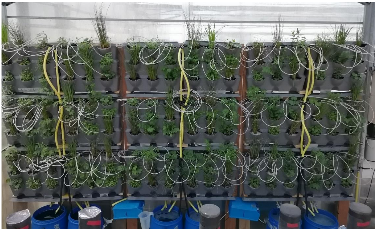
Figure 5: Green wall after the establishment period, on May 16, 2019. All specimens seemed to have adapted well to the greywater irrigation.
