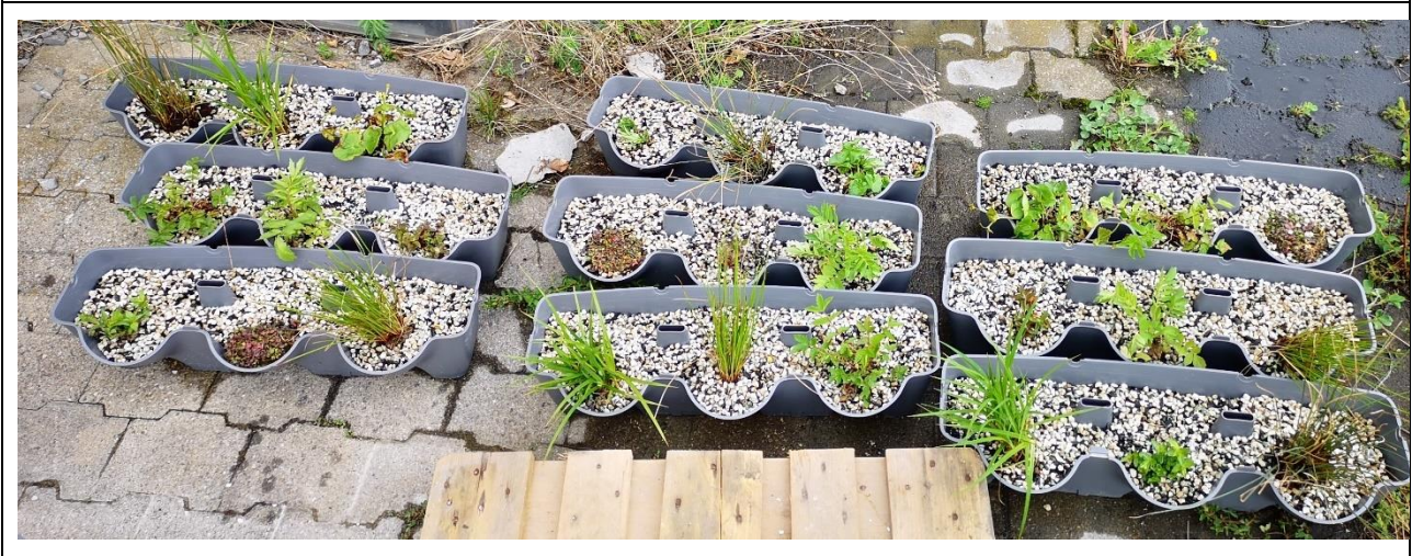
Figure 2: Sets horizontal elements after being planted and filled with the substrates. From top to bottom: Perlite/Coco, Vulkaponic, Vulkaponic/Biochar
