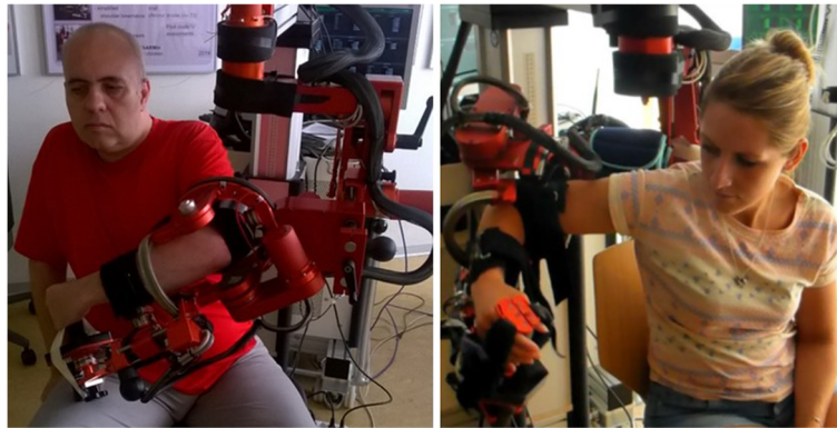
Fig. 3 Recording and replaying the QOM assessment. (Left) Stroke patient recorded while performing the QOM task in transparent mode. (Right) Participant in slave mode, experiencing the replayed QOM performance (mirrored to the participant’s dominant side)
