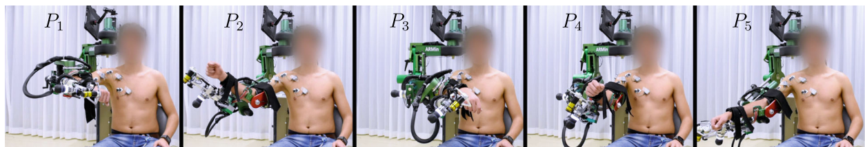
Fig. 2 The five EMG measurement poses ( P_1, \dots, P_5 ) for the efficacy comparison study: The poses represent the ADL usage of a stroke subject: P_1 ) Mouth and head reaching (-45,90,90,100,0), P_2 ) Ipsilateral reaching on shoulder level (-45,70,5,60,0), P_3 ) Contralateral reaching (10,70,30,40,60), P_4 ) Medial reaching at shoulder level (-15,65,15,50,0), P_5 ) Ipsilateral reaching on abdomen level (-50,55,30,40,0). Pose coordinates of the axes (1,2,3,4,5) in degree are according to anatomical axes definitions [39]. Axis 1 (horizontal shoulder abduction/adduction), axis 2 (shoulder elevation), axis 3 (internal /external shoulder rotation), axis 4 (elbow flexion/extension), and axis 5 (forearm pronation/supination). P_1 and P_2 are the chosen estimation poses (14,20) of the sensitivity analysis and P_3, P_4 and P_5 complement the workspace for stroke patients in ARMin. All coordinates of the poses of the sensitivity analysis and efficacy comparison study are shown in the Additional file 2
