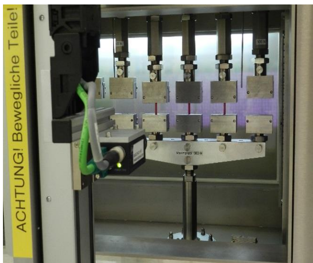
Fig. 2. Creep test setup in TFA including CCD video camera system for measuring creep strains.
