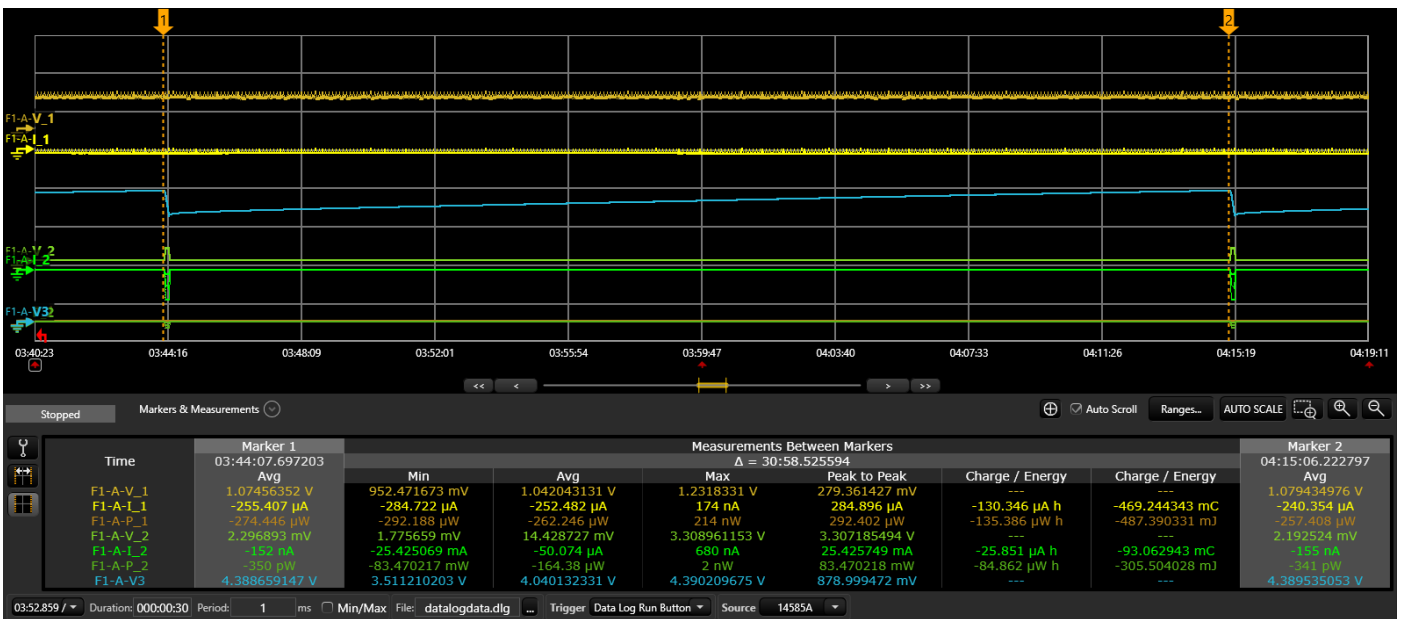
Figure 4. Zoom on a longer harvesting cycle (illuminance low). Harvest cycle duration is about 1846 seconds
