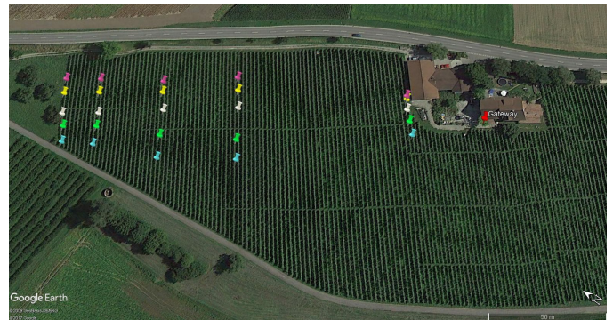
Fig. 3. Placement of gateway and nodes in the field
