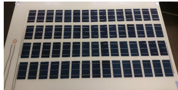
Figure 3: The picture shows the PV module with 60 half-cells and the integrated planar coil.
