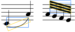
Fig. 3: Two examples of slanted symbols with their corresponding orthogonal bounding boxes (blue) and oriented bounding boxes (yellow). Orthogonal bounding boxes contain a significant amount of background pixels (left) and can have ample overlap with other bounding boxes (right). Oriented bounding boxes reduce these issues.
