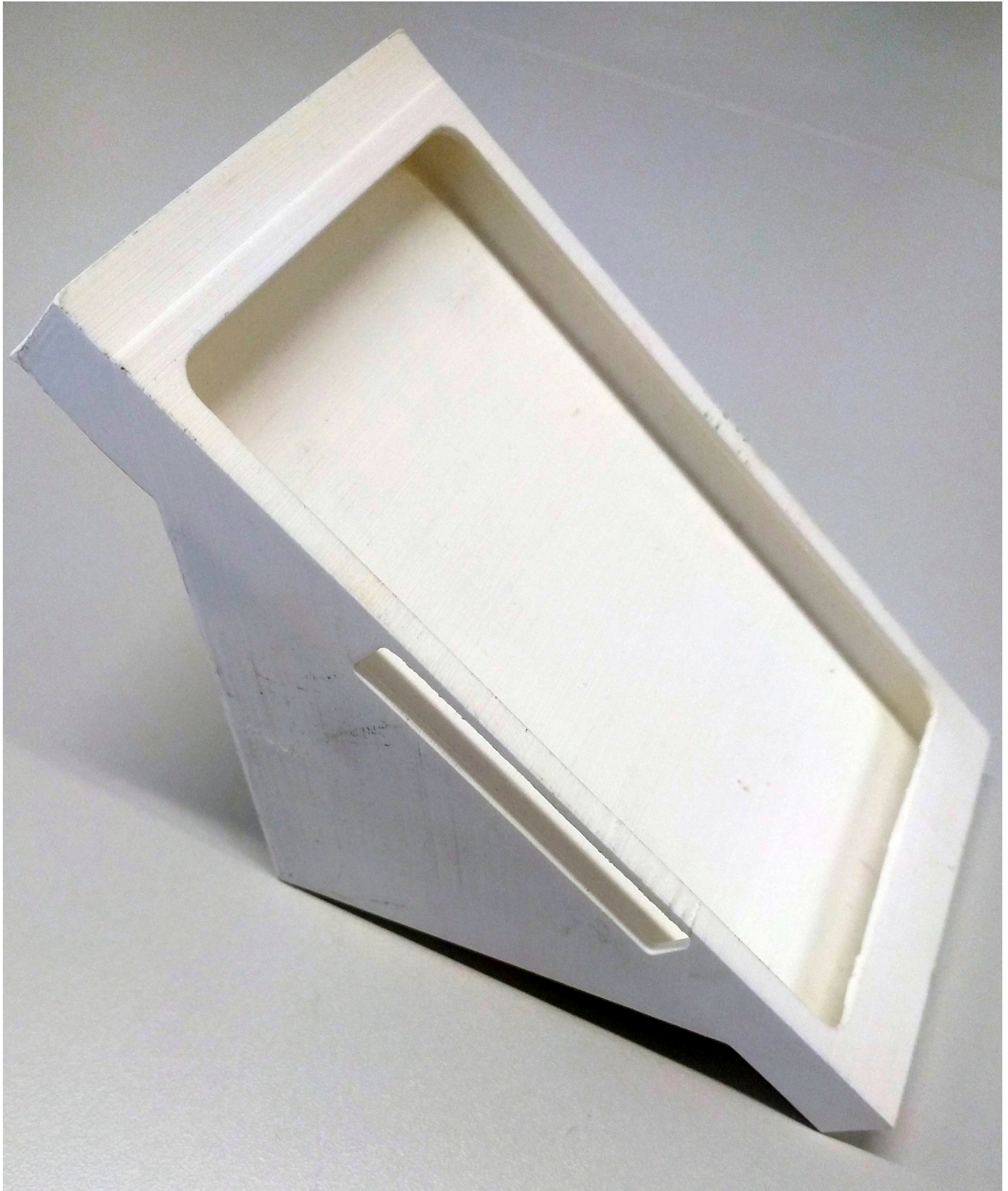
Fig 1. Measuring equipment. 3-D printed Smartphone Holder.
