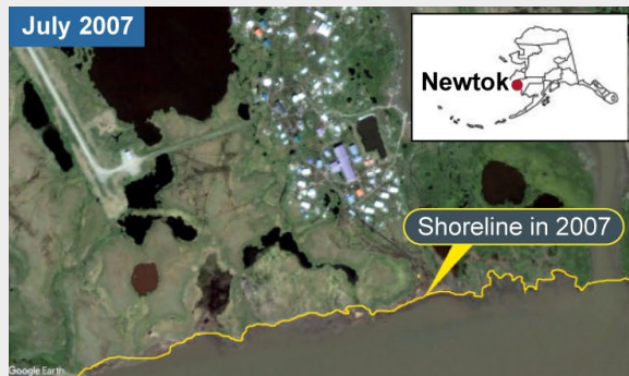
Figure 6: Shoreline erosion at Newtok, Alaska
