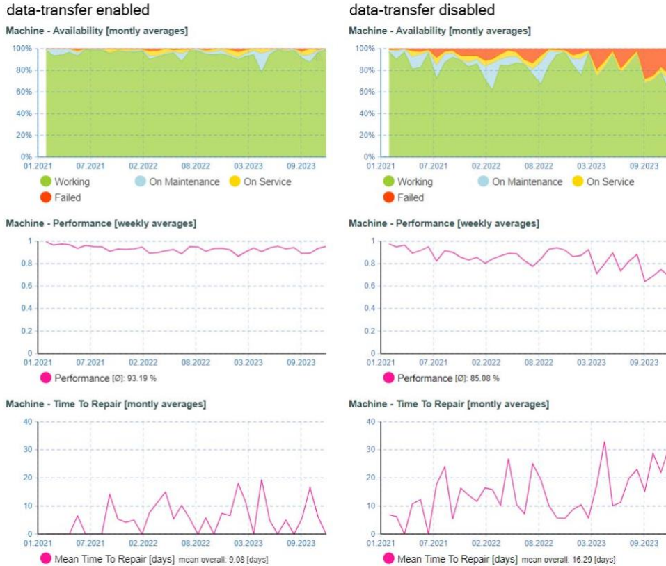
Fig. 5. Comparison of enabled (left) and disabled (right) data-sharing of a single simulation run in the demonstrator. The time stack chart on top shows the monthly averages of states of all machines of the installed base, the line chart in the middle shows the weekly average performance and the line chart at the bottom shows the monthly average time to repair or downtime of machines.
