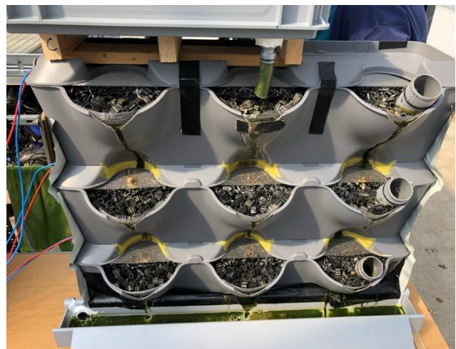
Figure 16: Wall B with Seramis expanded clay as reactor medium (reactors B1, B2, B3 from top to bottom)
