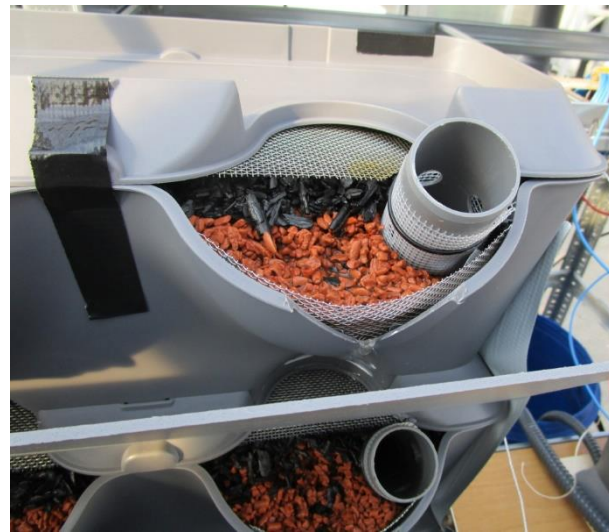
Figure 18: Detailed view of a measuring tube (Reactor B1) to monitor abiotic parameters in the anaerobic zone
