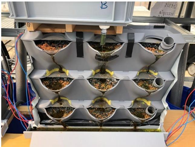
Figure 17: Wall C with HDPE biocarriers as reactor medium (reactors B1, B2, B3 from top to bottom)
