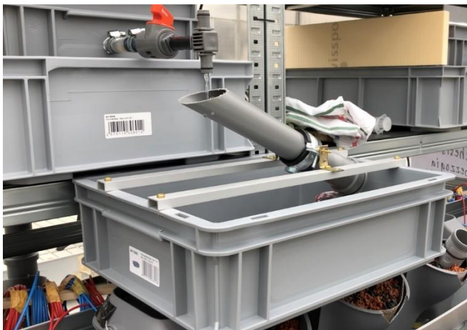
Figure 19: Detailed view of the mechanical dosing apparatus of Wall B, modeled after a Shishi-odoshi
