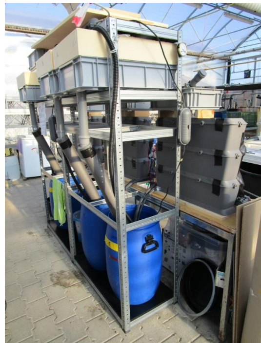
Figure 20: Rear view of the plant with the collection tanks at the top and the return pipes to the reservoirs (blue barrels) at the bottom
