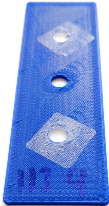
Figure S2. Sample holder (printed in blue PLA for the purpose of this visualization) with paraffin sections applied to two holes.
