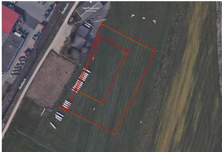
Figure 3 Rectangular flight tracks on the glider airfield in Winterthur. The green line shows the GBAS solution using a smoothing time constant of 10 s, the red line shows the SBAS solution.
