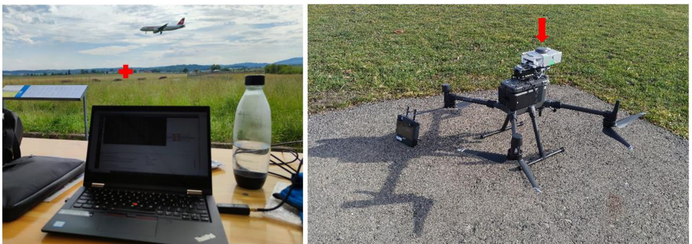
Figure 1 Left: GBAS VDB message recording at Zurich Airport, GBAS transmit antenna location is marked with red cross; Right: DJI Matrice used for flight test in Winterthur. Red arrow shows GNSS antenna position and GNSS receiver mount.
