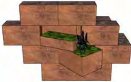
Figure 8: The oversized grip hole in the center provides space for medium-sized plants. This design leans to more structure in the facade with small crevices. Possible animals present: insects Substrate depth: 14-20 cm
