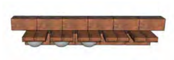
Figure 11: Two thin exposed bricks are clamped between two rows of bricks. In this case, these are custom-made (300×120×50 mm). Alternatively, a wooden board can be used. House martins use this board for their nests. Possible animals: House martins
