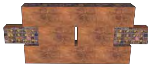
Figure 13: The module provides a gap that can be used by bats. In addition, two exposed stones are turned upside down and serve as an insect hotel. For this purpose, small plant stems are placed in the holes of the exposed stone. Possible animals present: insects, spiders, wild bees, bats
