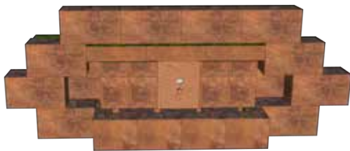
Figure 12: The element contains a nesting box (180×240×200 mm) for the redstart. The nest is protected by a cut wooden board and offers access by means of an oval entrance hole (200×32 mm). Possible animals: Redstart, other birds
