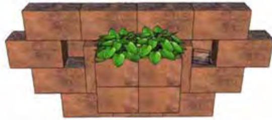
Figure 9: The exposed bricks are placed on top of each other, therefore doubling the substrate thickness. This element is particularly suitable for larger plants or plants that prefer wetter soils. Possible animals present: insects, spiders, snails, butterflies, small birds, sand lizards. Substrate depth: 27 cm.
