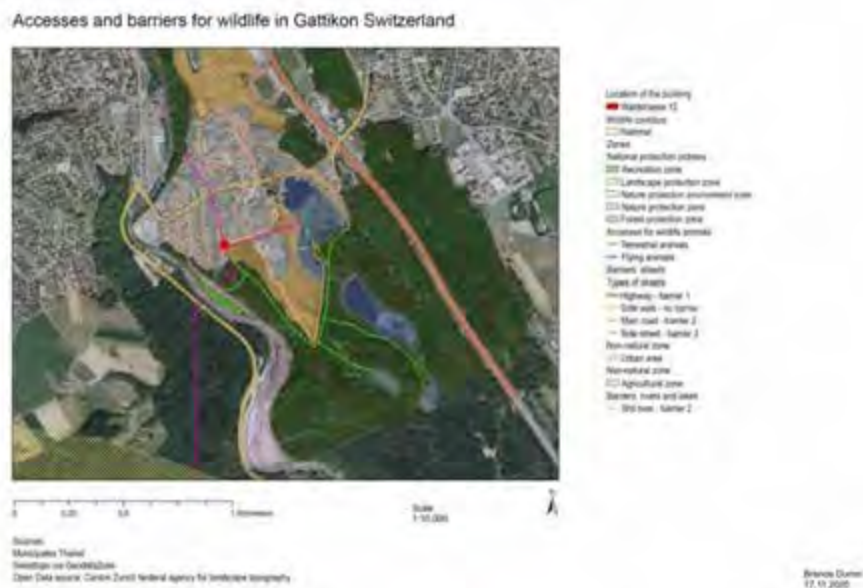
Figure 7: Barrier map created via ArcGIS; green lines show the access to the building available for ground-based animals, the purple lines the access for flying animals (Data from Zurich federal agency for landscape topography, 2017; municipality Thalwil, 2017)
