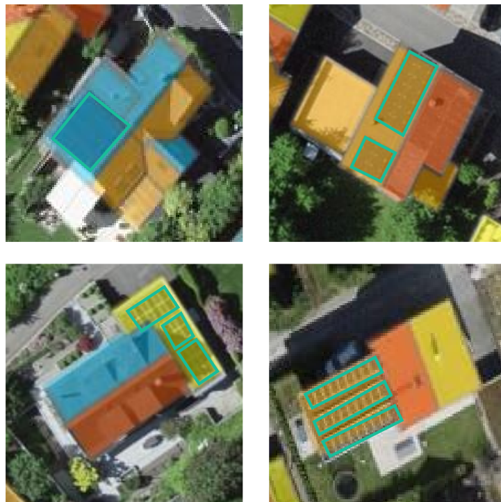
Figure 18: Excerpt of buildings with suboptimally placed PV panels detected by the model (categorized critical), green boundaries indicate existing PV panels
