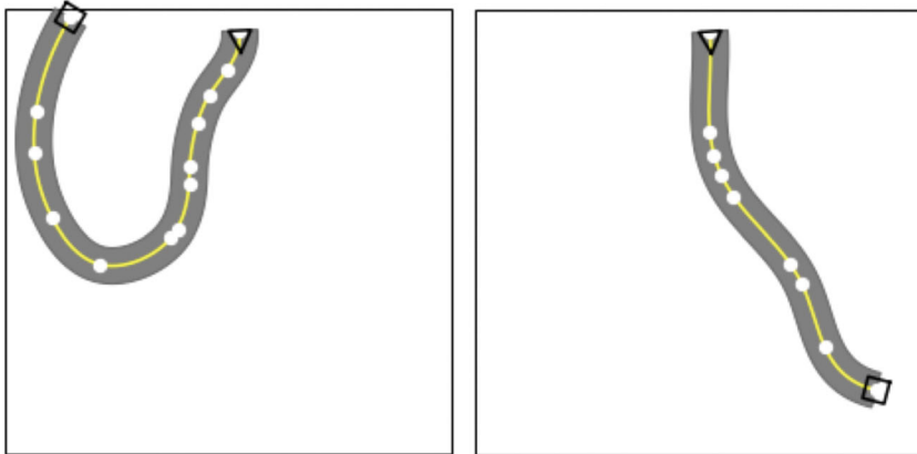
Fig. 1 Virtual roads for testing Lane Keeping systems. The white dots represent the road points, the (central) yellow lines represent the interpolated road spine, the triangles represent the starting locations, and the squares represent the target locations
