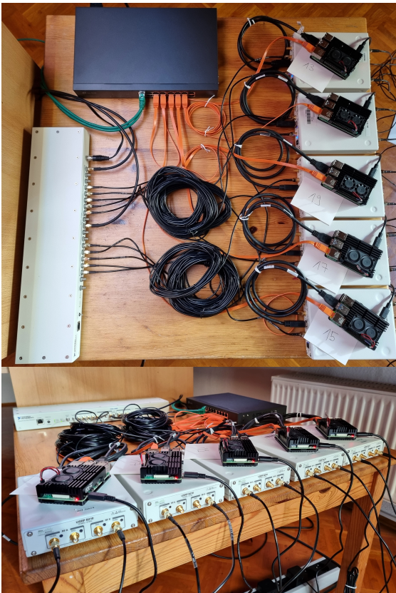
Fig. 2: Reference clock, network switch, TX SDRs and RasPis
