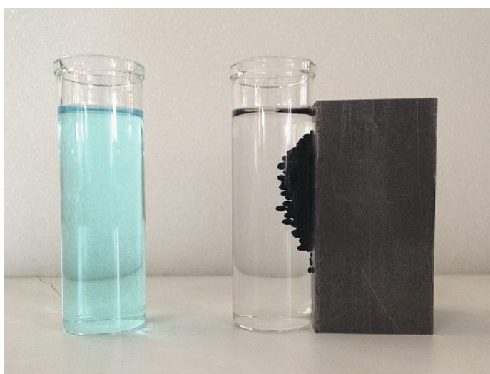
Fig. 7. Adsorption of \text{Cu}^{2+} ions on magnetic chitosan particles (left panel) and adsorption kinetics of \text{Pb}^{2+} on a commercial resin and on Laminaria digitata (marine algae) particles (right panel).
