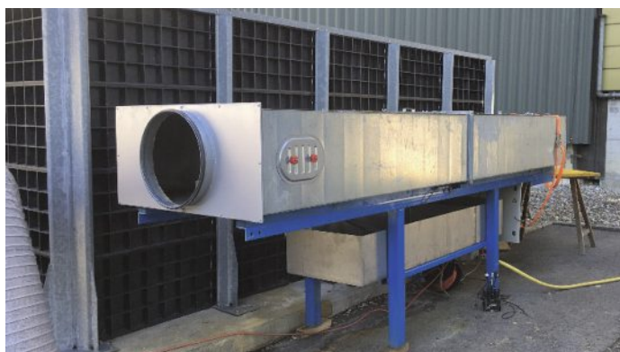
Fig. 3. Filtration prototype with a capacity of 5'000 m 3 /h connected to the air exhaust of the sewage sludge drying unit at the AVG (Abwasser Verband Glarnerland) plant of Bilten (GL).
