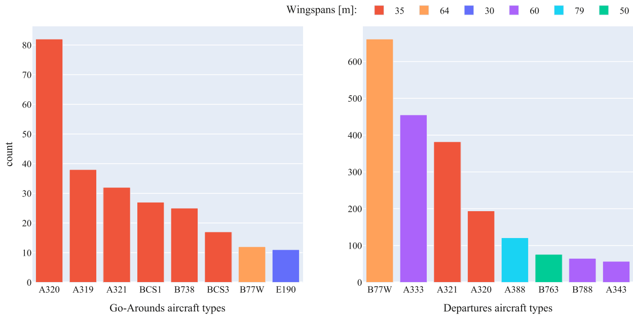
Fig. 5. The eight most commonly observed aircraft types flying go-arounds (left) and departures (right), and their associated wingspan. On runway 14, most of the GA are flown by narrow-body aircraft having an average wingspan of 34 m. Runway 16 is mostly used by wide-body aircraft with an average wingspan of 55 m.
