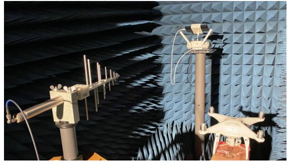
Figure 1: Recording of drone signals in the anechoic chamber. A DJI Phantom 4 Pro drone with the DJI Phantom GL300F remote control.
