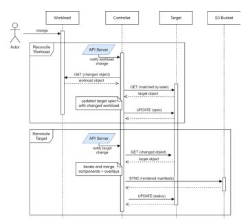
Fig. 5: Sequence diagram – Workload change
