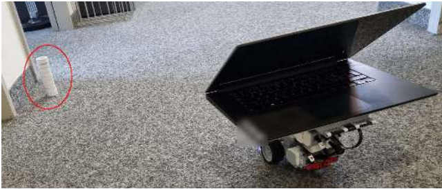
Figure 4: Robot driving to the circled beacon stack destination. The laptop acts as bluetooth receiver and edge voter.
