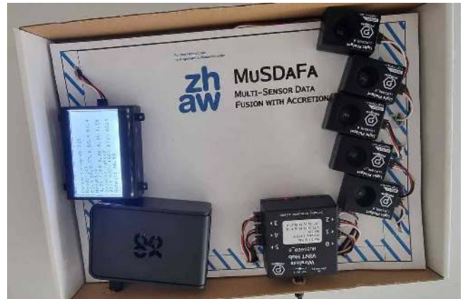
Figure 2: Portable 'shoe-box' testbed for our light sensor setup (Fig.1). A Raspberry Pi 4 runs the fusion script. An LCD display shows the voting results and weight values.
