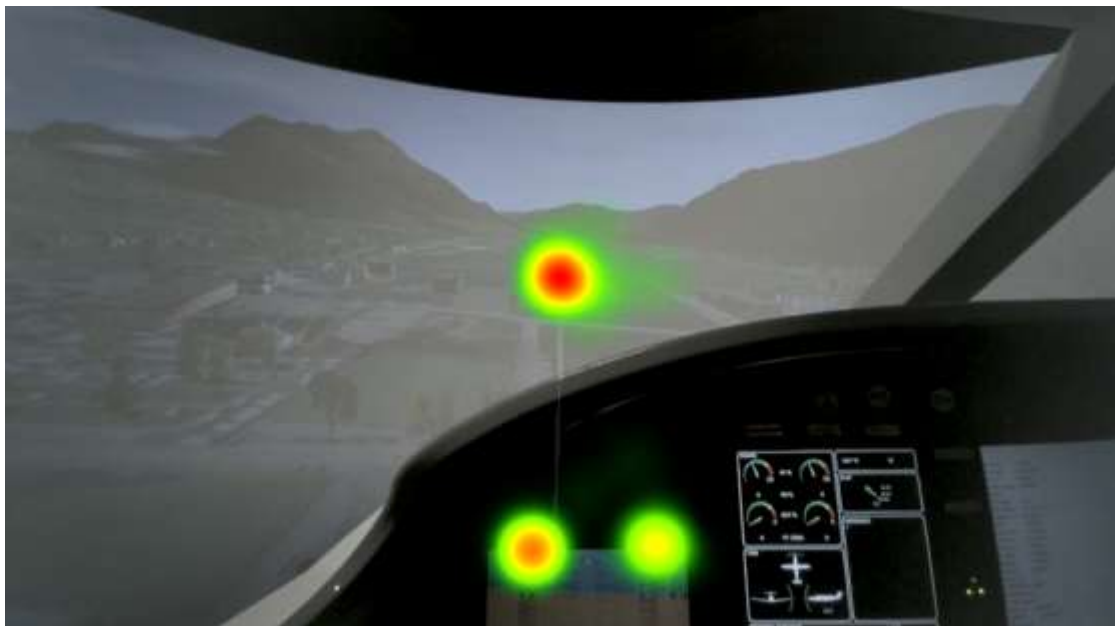
Figure 5: This is a heat map from the analysis of the eye tracking data in Tobii Pro Lab. The areas which have been looked at the most are marked in red. As it is visible, the main focus is on the runway, indicated by the red colour. The other focus lies on the speed indicator and then the vertical speed indicator.
