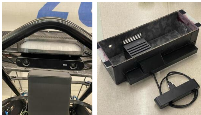
(a) The ZED mounted on the race car (b) The ZED together with the Jetson in the driverless box
