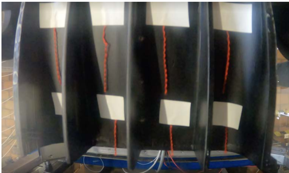
FIGURE 4.13: Attached flow in the diffuser
