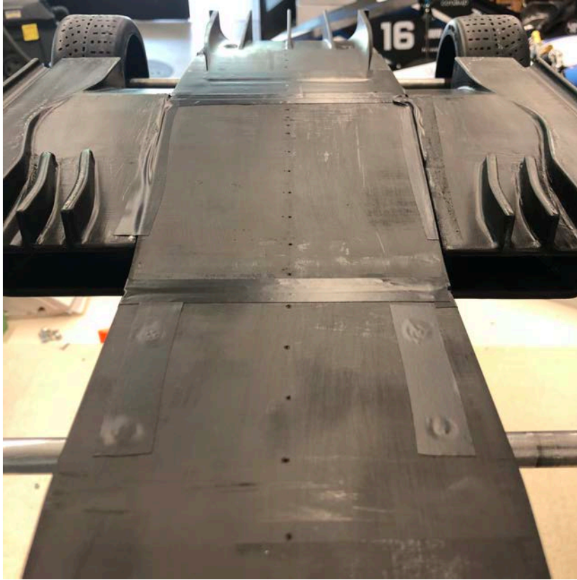
FIGURE 3.13: Static pressure ports on the underbody of the wind tunnel model
