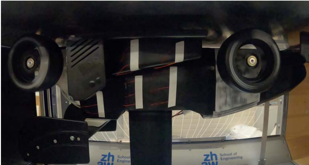
FIGURE 3.16: Short red tufts attached on the side of the wind tunnel model
