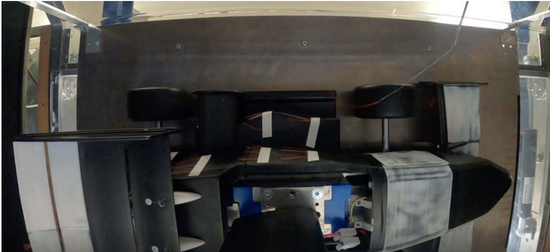
FIGURE 4.12: Flow on the side of the model
