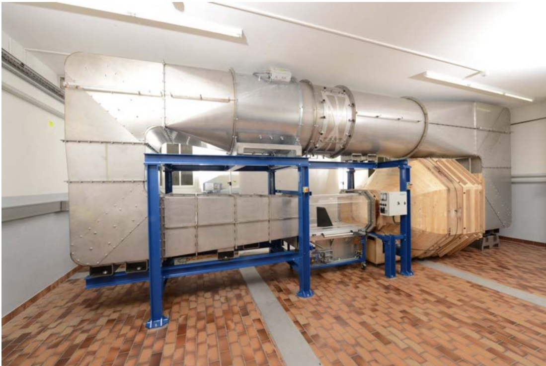
FIGURE 3.8: ALFA low speed wind tunnel of the ZAV [23]
