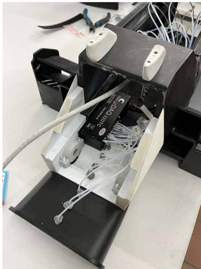
FIGURE 3.12: MicroDaq 32 Pressure Scanner connected to plastic hoses spread along the underbody and diffuser
