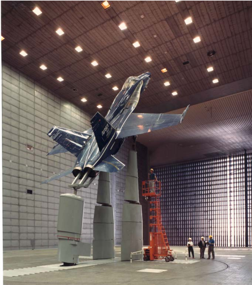
FIGURE 2.9: Full-scale F/A-18 fighter aircraft undergoing high angle of attack (AOA) wind tunnel tests at NASA's Ames Research Center [11]
