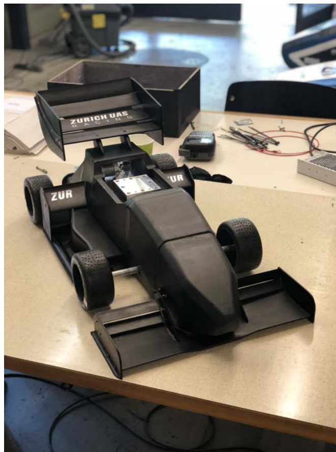
FIGURE 3.7: Fully assembled wind tunnel model
