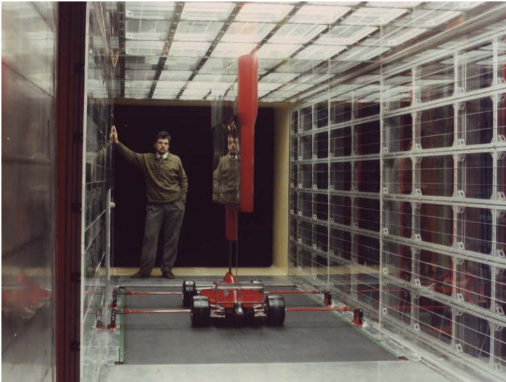
FIGURE 2.11: Scale model of a Formula 1 car in a wind tunnel with moving belt, courtesy of Mr. Marco Giachi, standing in the picture
