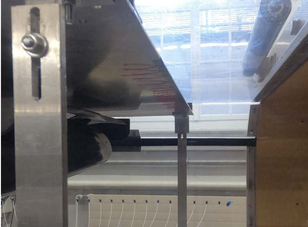
FIGURE 4.14: Tufts at the leading edge of the plate
