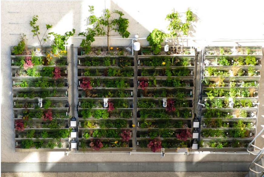
Fig. 28.3 Vertical greening system at the University of Natural Resources and Life Sciences Vienna (BOKU), Vienna, Austria. The system has a total size of 6m x 4m and consists of four individual systems with their own irrigation system. Monitoring included air and substrate temperature, substrate water content, precipitation, solar radiation, irrigation water volume and system output [13]
