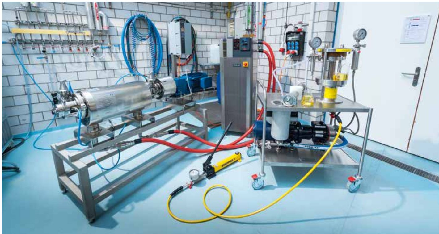
Test equipment for continuous filtration and quality stabilisation of deep-frying oil – an ILGI project. Photo: Frank Brüderli
