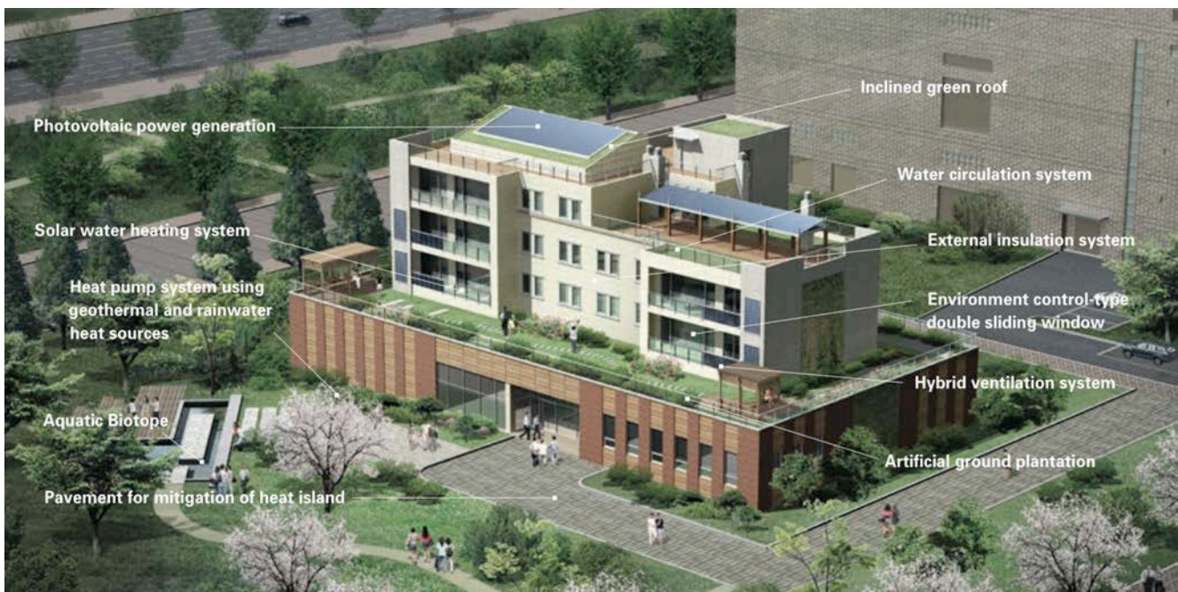
Figure 10. Isometric view of greenhome plus with indication of the main building integrated features for greening, water and energy management, and renewable energy production.
