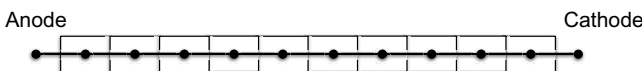
FIG. 2. Illustration of the spatial discretization. The grid consists of n+1 grid points which results in n-1 boxes.
