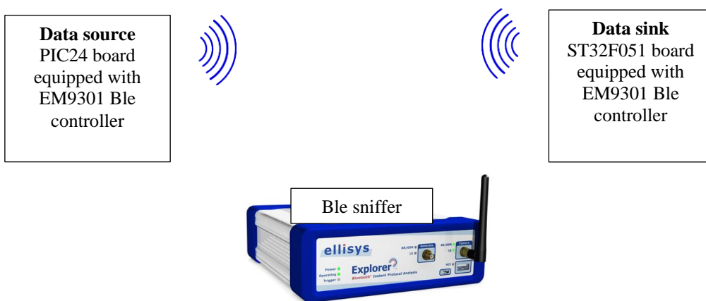
Fig.3 Setup to stream data and measure throughput rate
