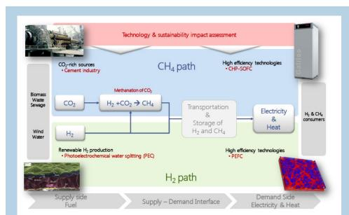
**Key:** carbon dioxide [CO<sub>2</sub>]; methane [CH<sub>4</sub>]; hydrogen [H<sub>2</sub>]; proton exchange membrane fuel cells [PEFCs]; combined heat and power [CHP]; solid oxide fuel cells [SOFCs].
