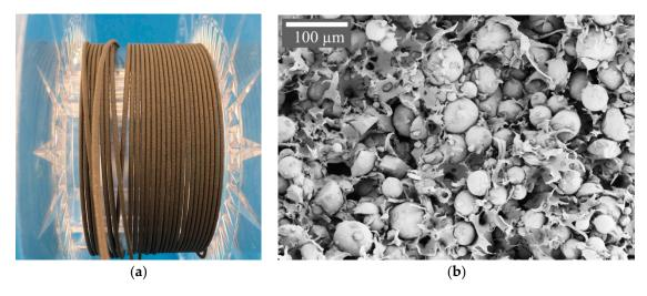
**Figure 2.** (a) Polymer-bonded magnetic filament flexible enough to be spooled on a standard filament spool with a diameter of 10 cm; (b) SEM micrograph of the extruded polymer-bonded magnetic compound, NdFeB particles inside the POM/PA12 matrix.
