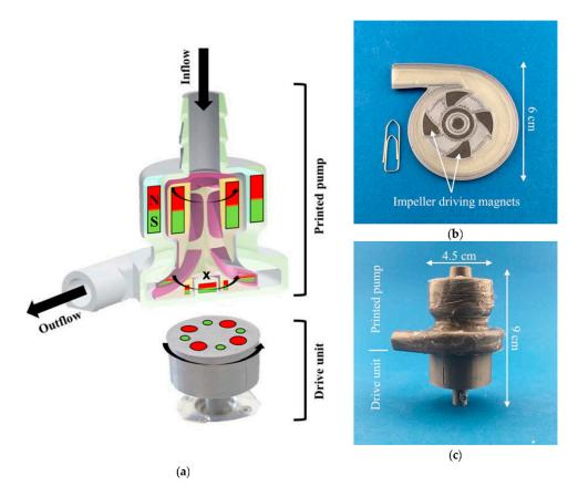
**Figure 1.** (a) Design scheme and coupling of the printed pump with integrated driving and bearing magnets in the housing and impeller; (b) Cross-section of the printed pump showing the used materials in different colors (silver: PLA, black: magnetic compound, beige: water-soluble BVOH); (c) Fully printed pump with drive unit after removal of support material (no magnets visible, coated with silicone).
