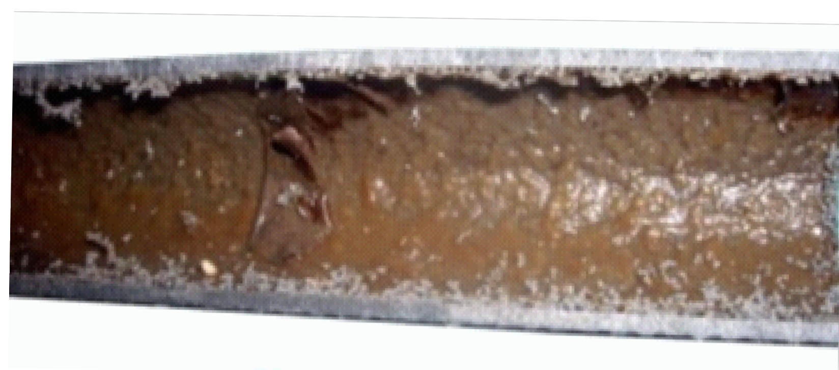
A cross-section through a water tube with biofilm.
